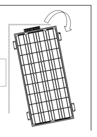
NOTE: Orient panel in level/plumb layout as desired before fixing in position.
