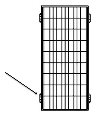
NOTE: Begin new fastener at indicated location first to secure panel in level plumb/level layout.
