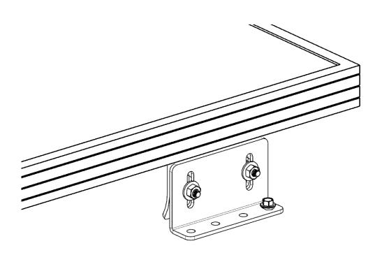
NOTE: Orient panel in level/plumb layout as desired before fixing in position.
